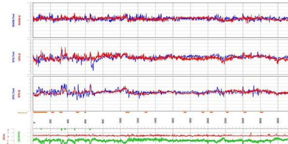
VIRTUAL RUN: A blind test in a horizontal well from the Permian basin demonstrates that QDrill sonic and density logs (red) are within the normal repeatability of conventional logging tools (blue). Photo: Quantico
